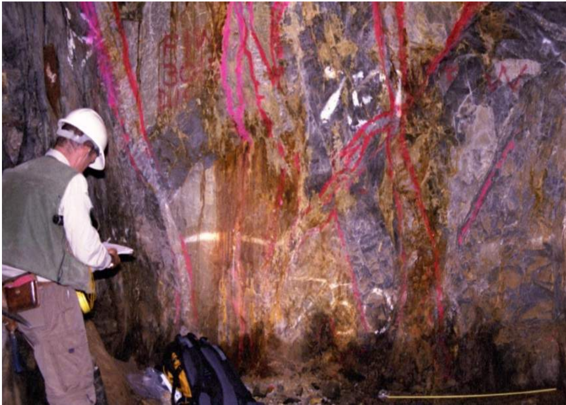
Figure 4. A shear-hosted quartz vein array exposed by recent underground exploration in the Challenger deposit, Adelong. Individual mineralised zones/veins are outlined in red. Photo: P. Downes, 2003.
